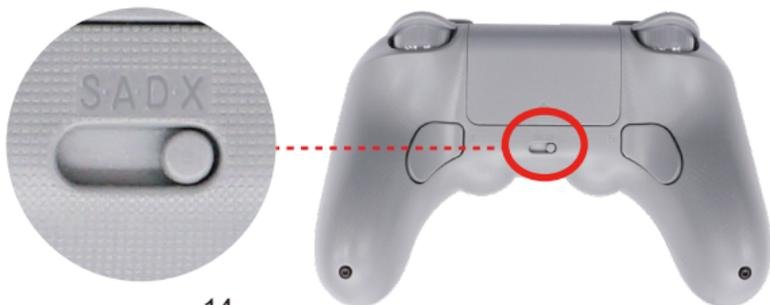
3) Press and hold "SYNC" button until LED starts flashing back and forth.
